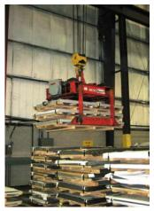
Sheet lifters handle single or multiple bundles of metal sheets or plates. They are operated by a hand wheel, chain wheel, electric motor or hydraulic cylinders. They can be equipped with low headroom designs; end hooks; telescoping carrying arms, adjustable load forks and much more. All lifters are engineered to order to exactly meet your requirements
