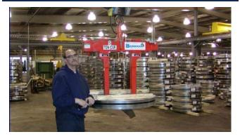
I.D. coil lifters are used to handle slit, banded coils from a packaging line and load onto pallets. Lifting pads are lowered through the I.D. and then opened to lift from under the coil. These lifters are operated by either a hand wheel or through an electric motor.
