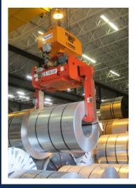
Motorized coil grabs are a fast, efficient way to handle coils. Features include low headroom designs, replaceable wear bars for high duty cycle operation, optical sensors, full length coil sensing flapper assemblies on drop legs, protective padding and rollers, special bail configurations, motorized rotation and built-in weigh scales.
