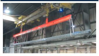
Whether lifting 30 pounds or 300 tons, Bushman designs spreader beams with optimum strength-to-weight ratios so that your crane can lift the maximum live load.
