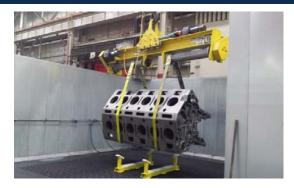
The FLIP-RITE® material handling system allows safe raising, lowering, rotating and leveling of large, bulky or oddly shaped objects up to 100 tons. The FLIP-RITE® gently rotates your load within the envelope of conventional lifting straps without the shock loading and wear & tear to your crane when attempting to flip over heavy loads.
