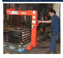
Bushman pallet lifters are available in capacities from 500 pounds to 20 tons. Pallet lifter features include:
