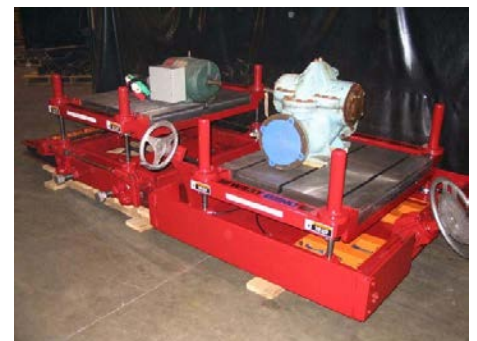
Independently adjustable dual-table pump test stand
