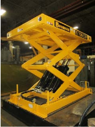
30,000 pound capacity two-high hydraulic scissor lift.
