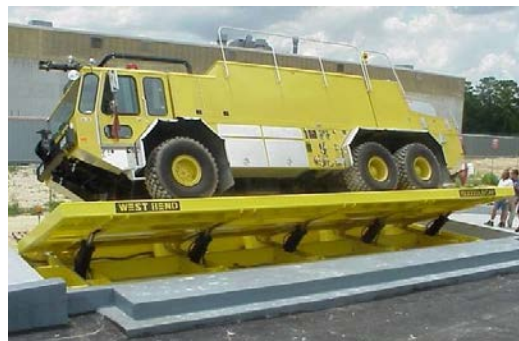
150,000 pound capacity rescue vehicle hydraulic tilt-test platform
