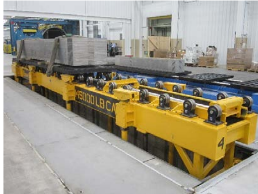
145,000 pound capacity pit-mounted electric jack screw lift,
