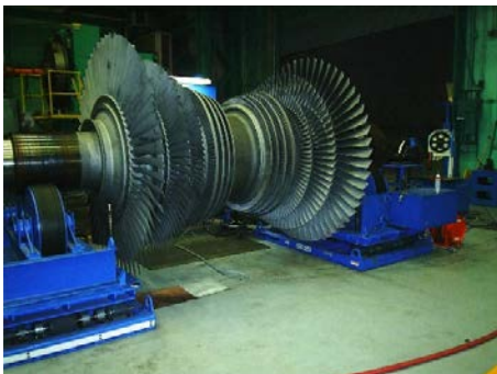
120,000 pound capacity portable electric screw arbor lifts on air bearings
