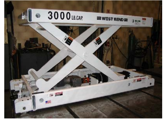
3,000 pound capacity electric screw powered mobile scissor lift table.
